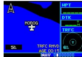
Thumbnail Traffic displayed on the GNS 430W. NOTE: The thumbnail will display traffic coasting "TRFC CST" or traffic removed "TRFC RMVD" in the lower right when TIS messages have been missed.
