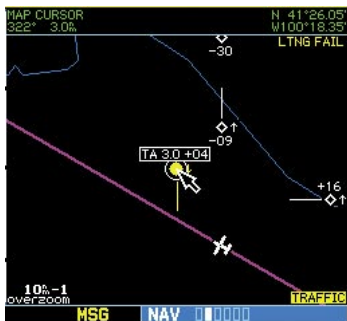
Displaying traffic range and altitude separation using the Map Panning feature.
