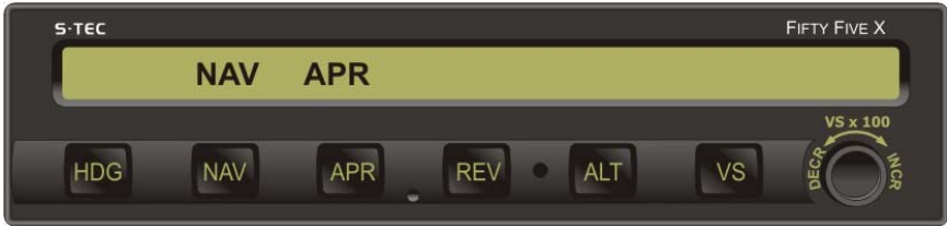
Fig. 3-7. AP Display, APR Mode Engaged
