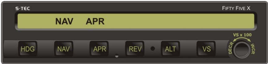
Fig. 3-33. AP Display, APR Mode Engaged, Track LOC Back Course Outbound
