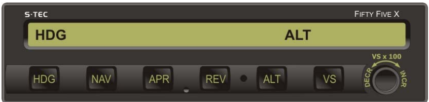
Fig. 3-21. AP Display, HDG and ALT HOLD Modes Engaged
