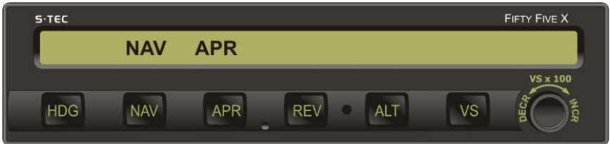
Fig. 3-41. AP Display, APR Mode Engaged, Track LOC Front Course Inbound
