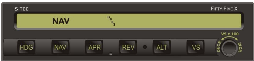
Fig. 3-10. AP Display, GPSS Mode Engaged
