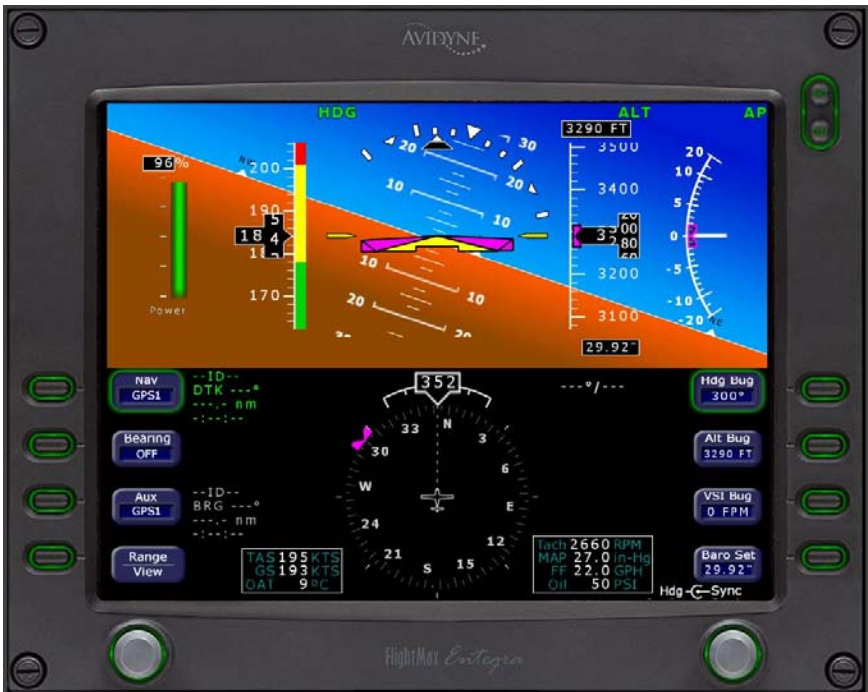
Fig. 3-46. PFD Display, HDG and ALT HOLD AP Modes Engaged
