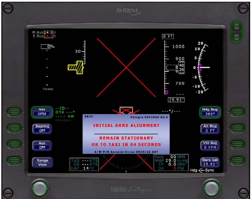
Fig. 2-3. PFD Display, INITIAL AHRS ALIGNMENT Message
