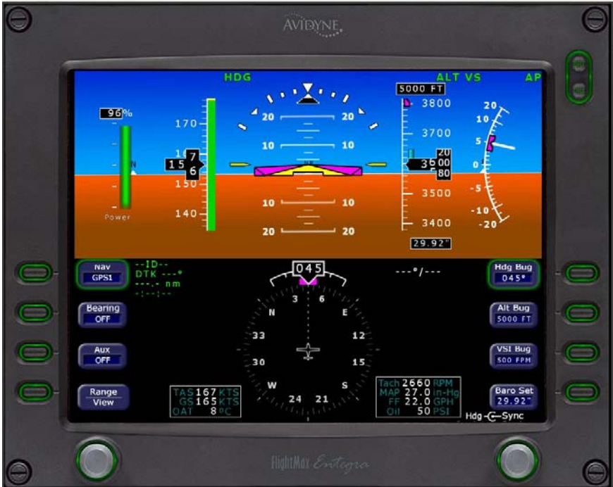
Fig. 3-20. PFD Display, HDG and VS Modes Engaged, ALT HOLD Mode Armed
