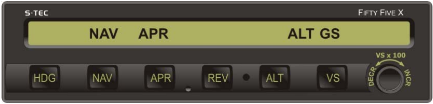
Fig. 3-25. AP Display, NAV, APR and ALT HOLD Modes Engaged, GS Mode Armed
