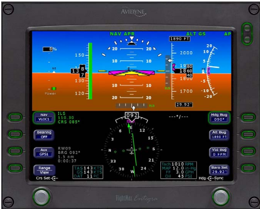
Fig. 3-26. PF-D Display, NAV, APR, and ALT HOLD Modes Engaged, GS Mode Armed
