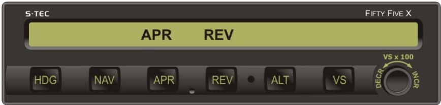
Fig. 3-30. AP Display, APR Mode Engaged, Back Course
