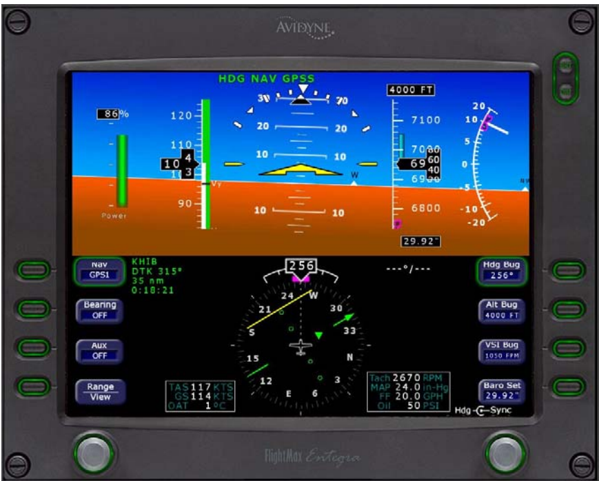
Fig. 3-13. PFD Display, HDG Mode Engaged, GPSS Mode Armed
