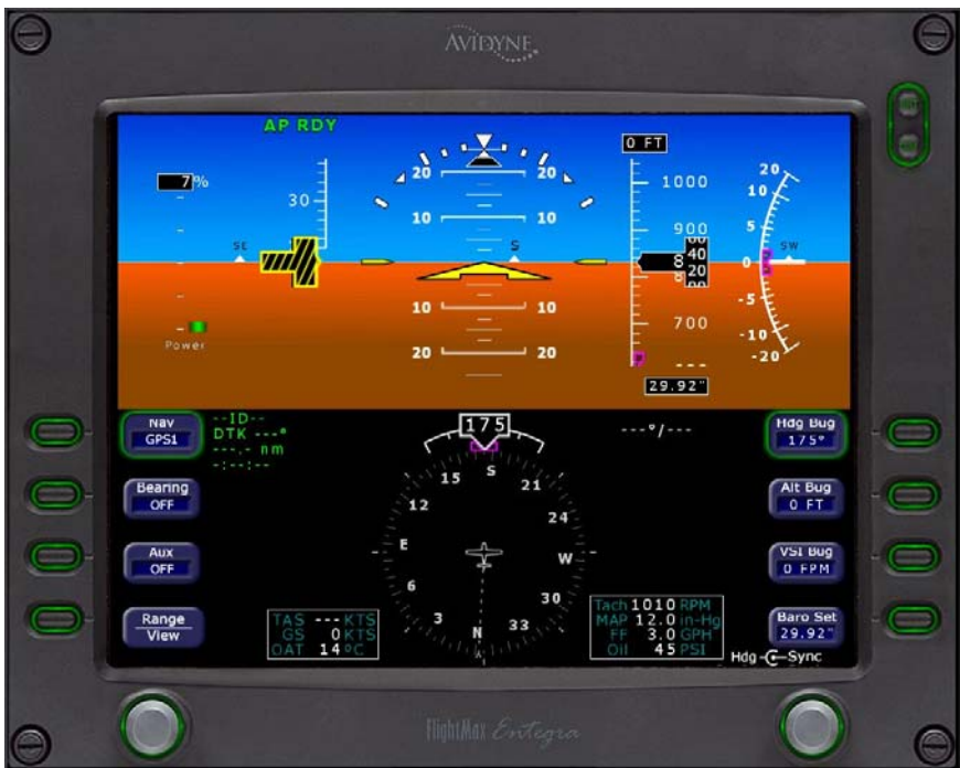
Fig. 2-5. PFD Display, AP RDY Annunciation
