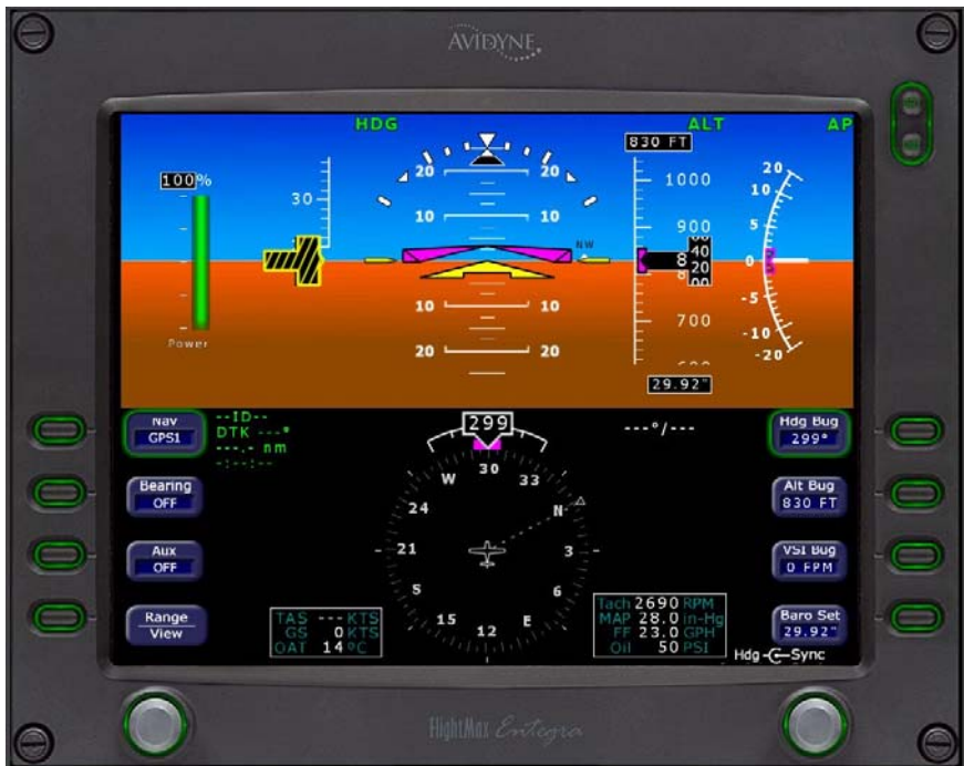
Fig. 2-11. PFD Display, HDG and ALT HOLD Modes Engaged (Pre-Flight)
