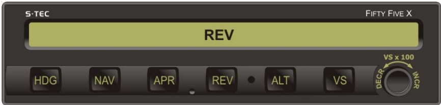
Fig. 3-43. AP Display, REV Mode Engaged, Track VOR Front Course Outbound
