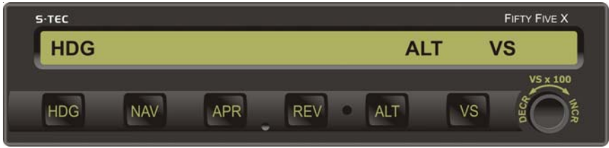
Fig. 3-19. AP Display, HDG and VS Modes Engaged, ALT HOLD Mode Armed
