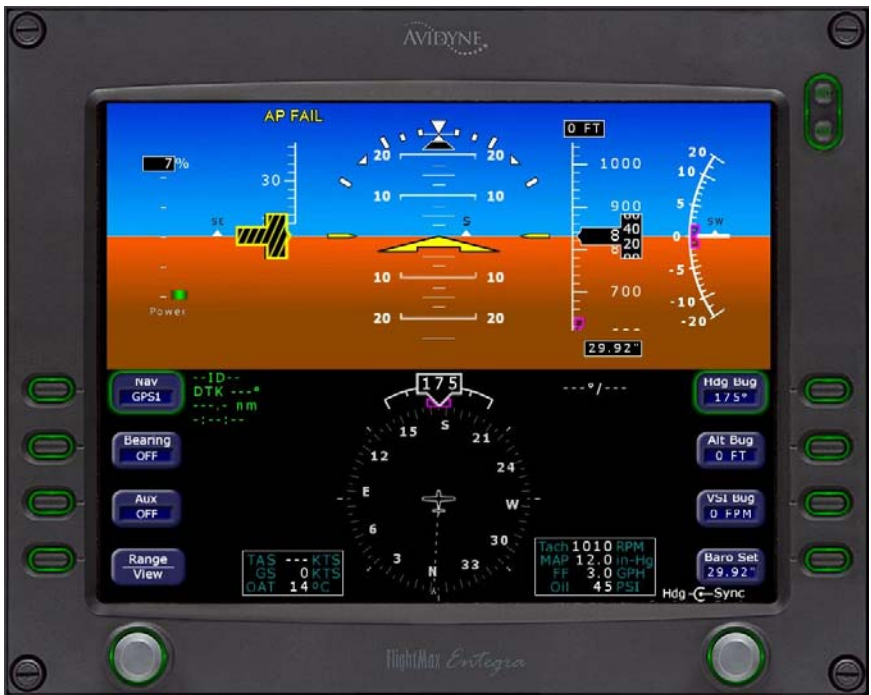
Fig. 2-7. PFD Display, AP FAIL Annunciation
