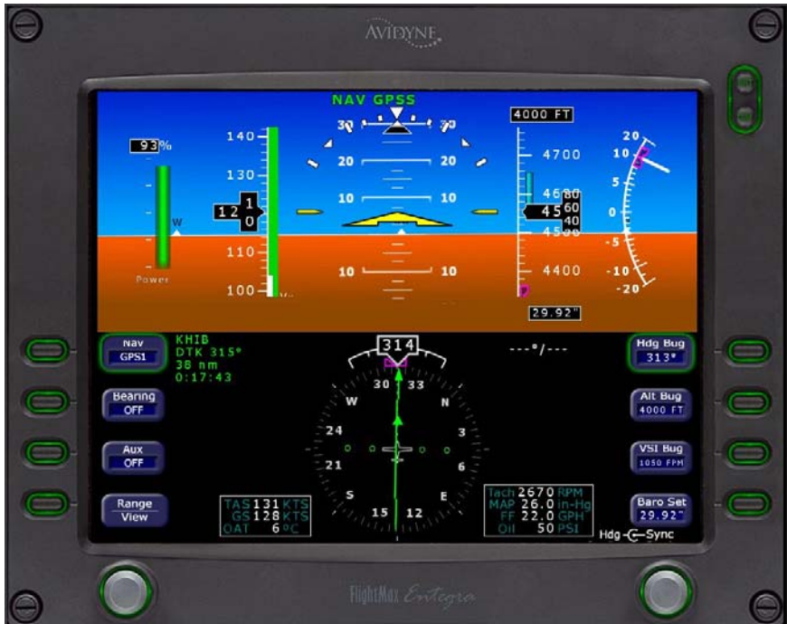
Fig. 3-11. PFD Display, GPSS Mode Engaged
