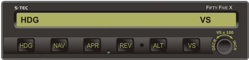
Fig. 3-16. AP Display, HDG and VS Modes Engaged
