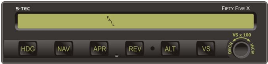
Fig. 2-6. AP Display, FAIL Annunciation
