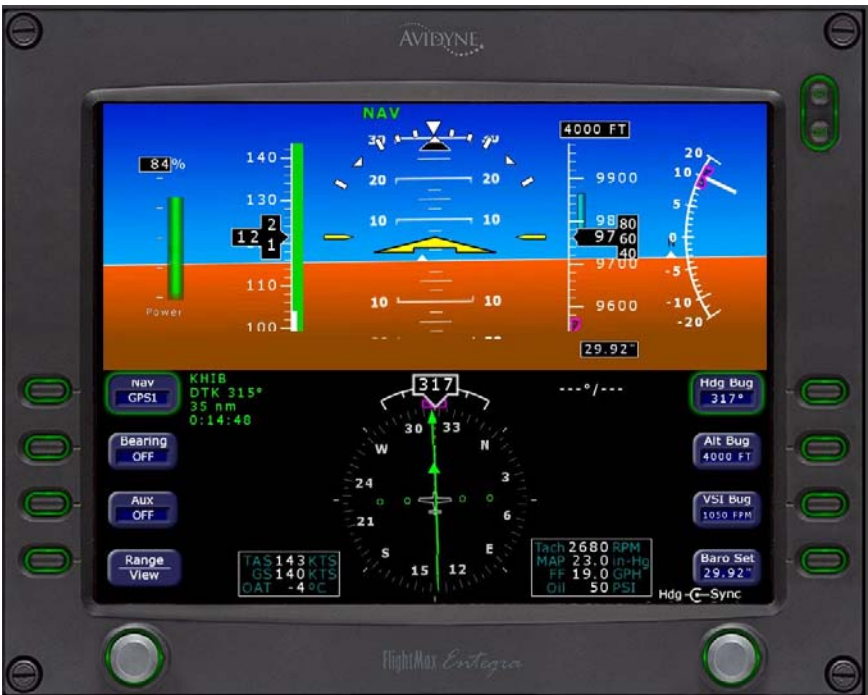
Fig. 3-6. PFD Display, NAV Mode Engaged, A/C Tracking Course
