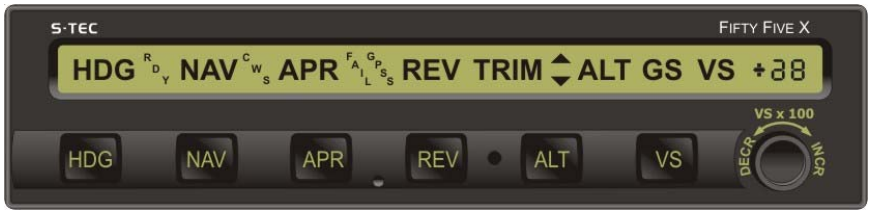
Fig. 2-1. AP Display, Power-Up Annunciations
