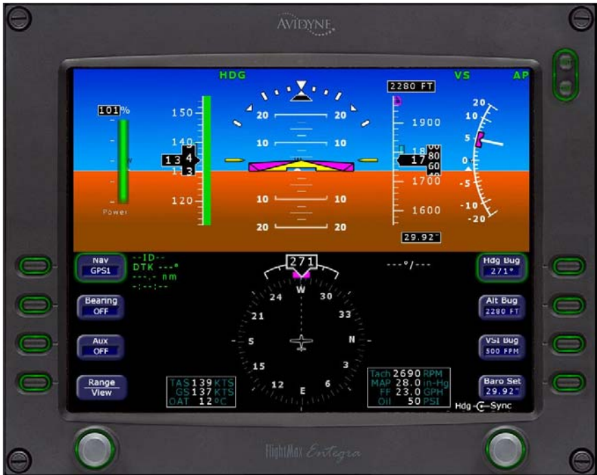
Fig. 3-17. PFD Display, HDG and VS Modes Engaged
