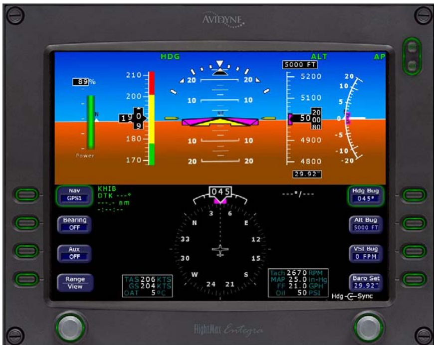
Fig. 3-15. PFD Display, HDG and ALT HOLD Modes Engaged
